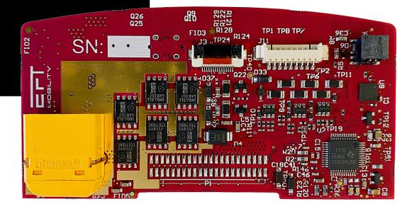
The EFT-BMS-14 (Battery Management System) is designed as a modular BMS platform that monitors and controls our UAV battery packs. It includes all relevant monitoring functions as well as control functionality.
