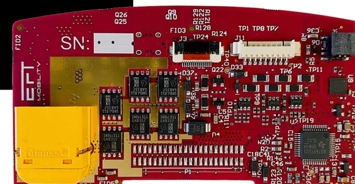
The EFT-BMS-14 (Battery Management System) is designed as a modular BMS platform that monitors and controls our UAV battery packs. It includes all relevant monitoring functions as well as control functionality.
